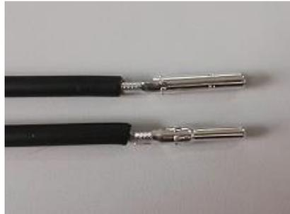
Third step: insert the metal core into inner of connector respectively. (Pay attention to do not
